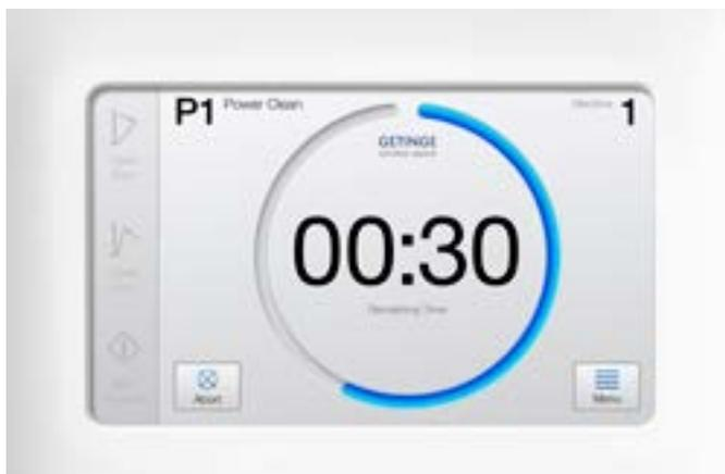
*CENTRIC provides status at a glance with clear information for each washer-disinfector – even from a distance.*
