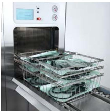
*Automatic loader and unloader for Baskets (GL64B).*
