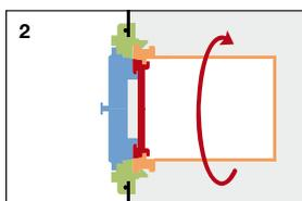
**Picture 2** shows the interlocking of the two units by a 60-degree rotation.
